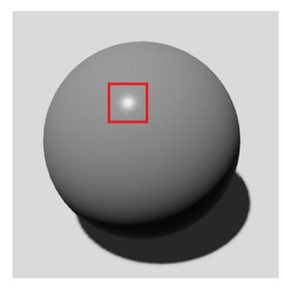
The specular color can be defined using a metalness map (which uses the diffuse color as a base color), or a specular map (the specular color is defined separately from the diffuse color).
