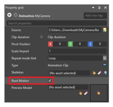
When root motion is enabled, Stride applies the **root node animation** to the <u>TransformComponent</u> of the entity you add the animation to, instead of applying it to the skeleton.
