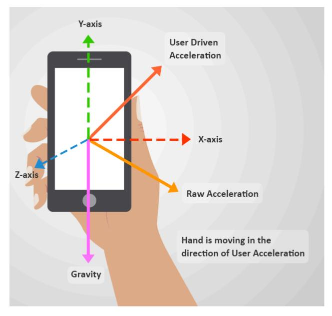
Motion sensors have a single field that specifies the current **acceleration vector** on the device. Stride measures the acceleration in **meters per second squared**.
