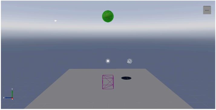
7. Let's make the trigger a larger area. In the **Property Grid**, under the **Transform** component properties, set the **scale** to: *X*:2, *Y*:2, *Z*:2
