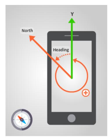
To get this angle, use <u>CompassSensor.Heading</u>. For example:
