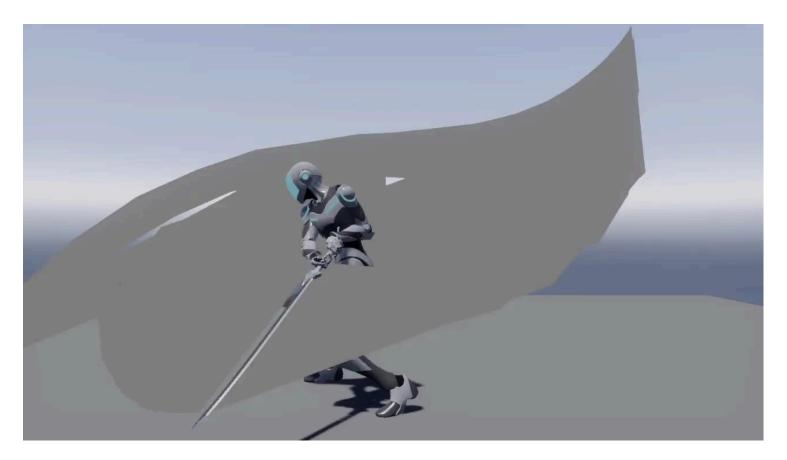
Rather than the particles connecting in order, the strip erratically jumps between particles. (This is the same problem alpha-blended quads have when they're not properly sorted.)
