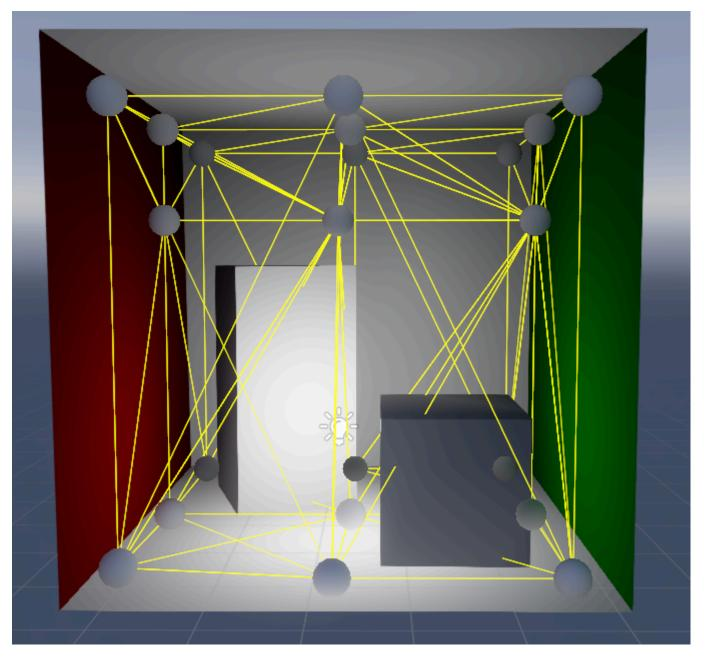
Stride colors pixels within a light probe area to simulate the effect of light bouncing from nearby surfaces. To find a color for a given pixel, Stride interpolates from the lighting captured by the four surrounding light probes.
