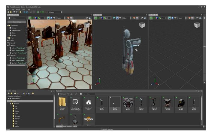
In the center pane, we already have a prefab named **Lamp**. In the right pane, we create a new prefab named **Boxes**, comprising several box entities positioned together. We add the Boxes prefab to the Lamp prefab. Changes made to the Boxes prefab are reflected in the Lamp prefab. These are in turn reflected in the instances of the Lamp prefab in the scene (left pane).
