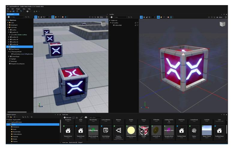
Just like with Unity<sup>®</sup>, in Stride, you can add prefabs to other prefabs. These are called **nested prefabs**. If you modify a nested prefab, all the dependent prefabs inherit the change automatically.
