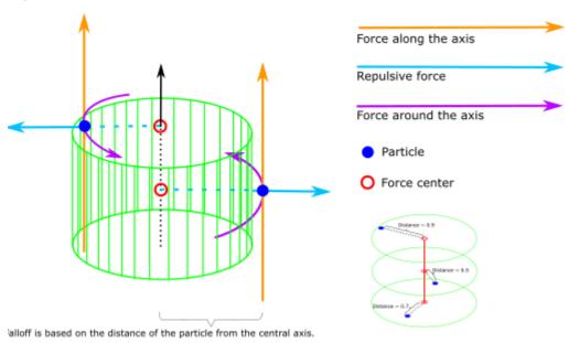
When the bounding shape is a cylinder, the falloff distance is based on the radial distance of the particle from the cylinder's local Y axis. The particle height (position on the Y axis) is ignored unless the particle is outside the cylinder, in which case the distance is always 1.
