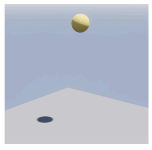
The Sphere (rigidbody) responds to gravity and falls. The Ground (static collider) breaks its fall. But there's no bounce effect yet.
