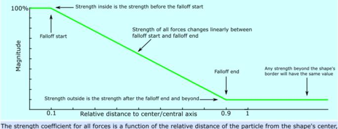
The strength coefficient for all forces is a function of the relative distance of the particle from the shape's cent with 1 being the shape's boundaries, and more than 1 being outside the shape.
