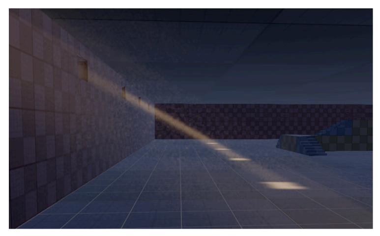
To reduce this effect, in the **light shaft component properties**, reduce the **density** and increase the **sample count**.
