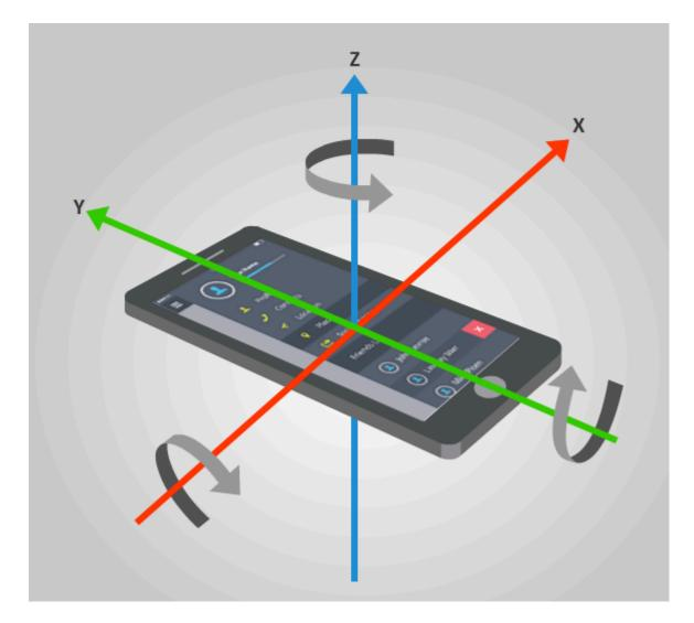
To get the rotation speed, use <u>GyroscopeSensor.RotationRate</u>. For example:
