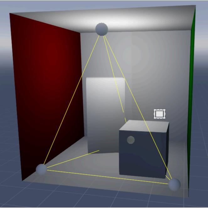
• At least one light probe must be on a different plane from the rest. For example, the probes in the screenshot below won't work, as they are on a flat plane and create no volume:
