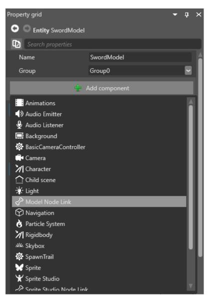
We can use this to link the SwordModel to a point in the mannequinModel skeleton. There's no need to specify a target, as the entity uses its parent entity (**mannequinModel**) by default.
