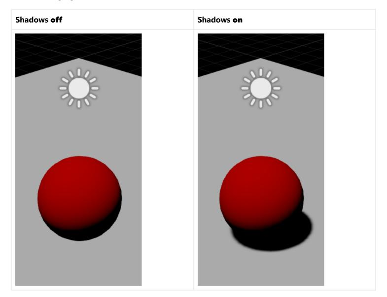
Only directional lights, point lights, and spot lights can cast shadows.
