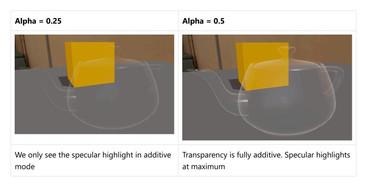
• If the **Alpha** <= 1.0, the material is semi-opaque with the diffuse/emissive component. If the diffuse component has an alpha, it's transparent.
