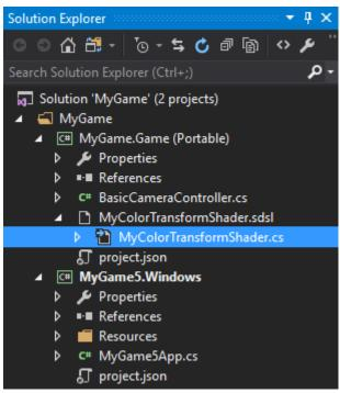
6. Open the .sds1 file, remove the existing lines, and write your shader.
