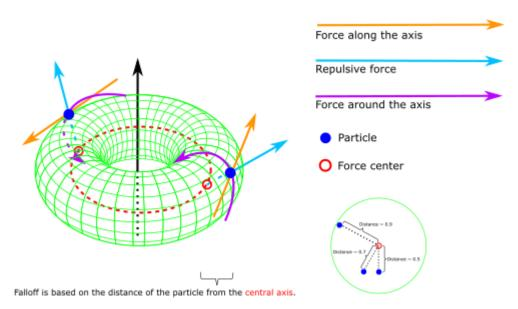
When the bounding shape is a torus, the field's nature changes completely. The falloff distance is based on the radial distance of the particle from the torus's inner circle (axis of revolution, shown in red), choosing a point on the circle closest to the particle.
